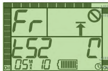
Figure A2-7: Helium confirmation screens at test 51, showing the alternating values of "HE" (for "Helium"; top), "Fr" (for "Fraction"; middle), and a numeric value (indicating the assumed fraction of Helium; bottom) for the diluent mixture.
