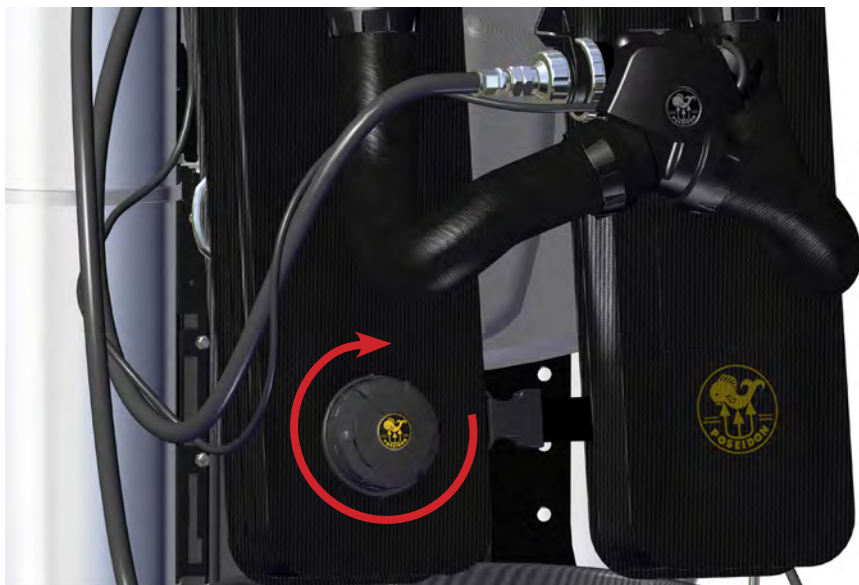
Figure 1-70. Make sure the OPV is in the maximum closed position.
