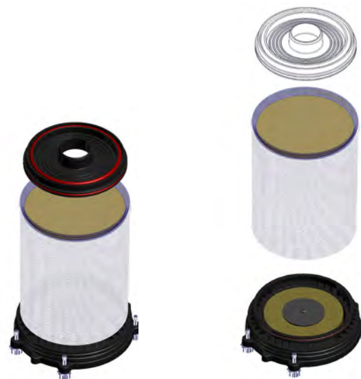
Figure 1-59. Remove the cartridge top plate.
