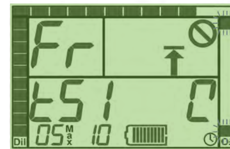
Figure A2-8: Oxygen confirmation screens at test 52, showing the alternating values of "O 2 " (for "Oxygen"; top), "Fr" (for "Fraction"; middle), and a numeric value (indicating the assumed fraction of Oxygen; bottom) for the diluent mixture.
