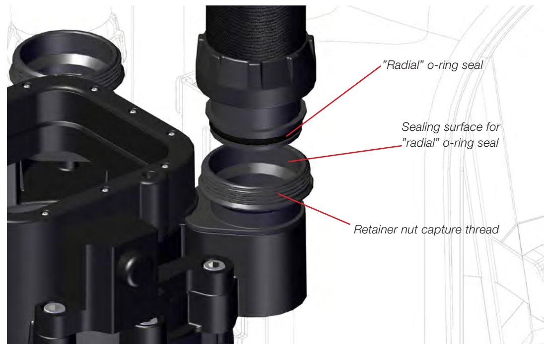
Figure 1-12. Typical “Radial” type o-ring seal.
