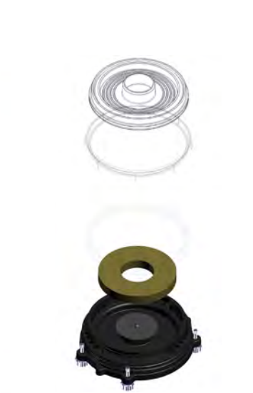
Figure 1-61. Lift and remove the lower sponge; inspect for collected water. Rinse, dry, and store the lower sponge; disinfect if desired.
