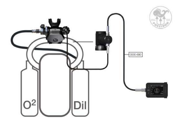
Non-Poseidon Rebreather: The M28 uses one cable (0000-690) to connect to the C-POD, using either a galvanic or a solid state as a third cell to act as back-up electronics on any non-Poseidon rebreather. A SE7EN BOV and HUD complement the system to provide greater functionality and ease of use.
