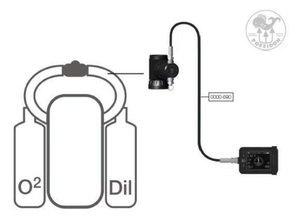
**Non-Poseidon Rebreather:** The M28 uses one cable (0000-690) to connect to the C-POD, using either a galvanic or a solid state as a third cell to act as back-up electronics on any non-Poseidon rebreather.
