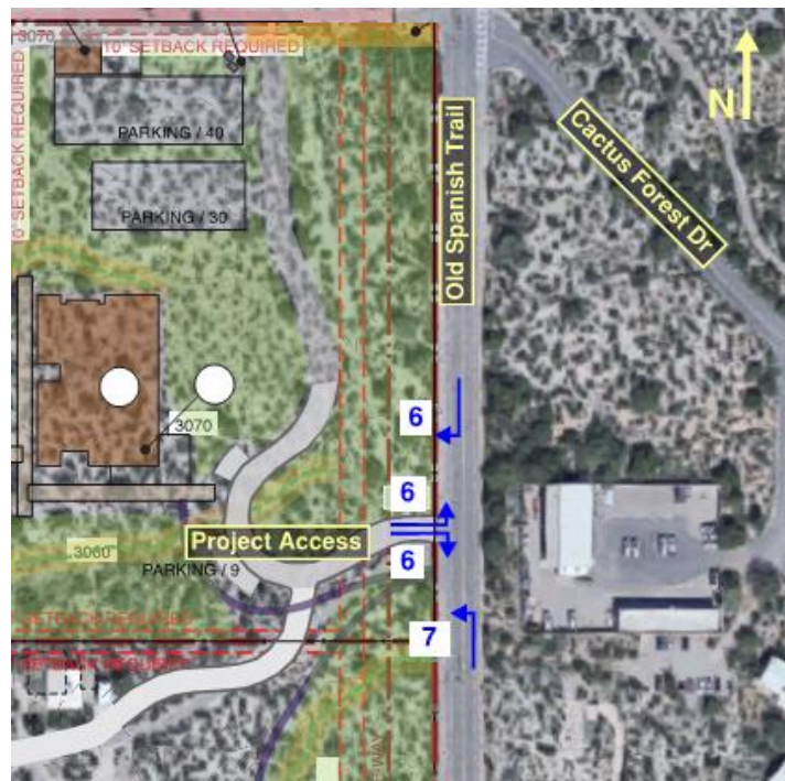
Figure 4. Project Access Turning Movements (PM Peak Hour)
