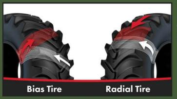
Radial tire construction lessens wheel tracking and compaction beneath sprinklers utilizing a wider face tread. The rugged radial tire design cuts maintenance costs by reducing flats in the field.
