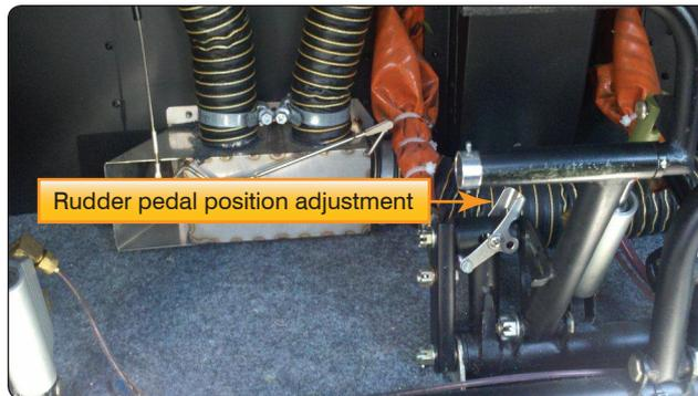
Figure 16-10. Adjustment lever for the rudder pedal position.
