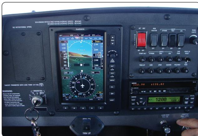
Figure 16-15. EFIS indication of level cruise flight.
