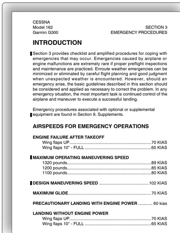
Figure 16-16. Example of a POH Emergency Procedures section.
