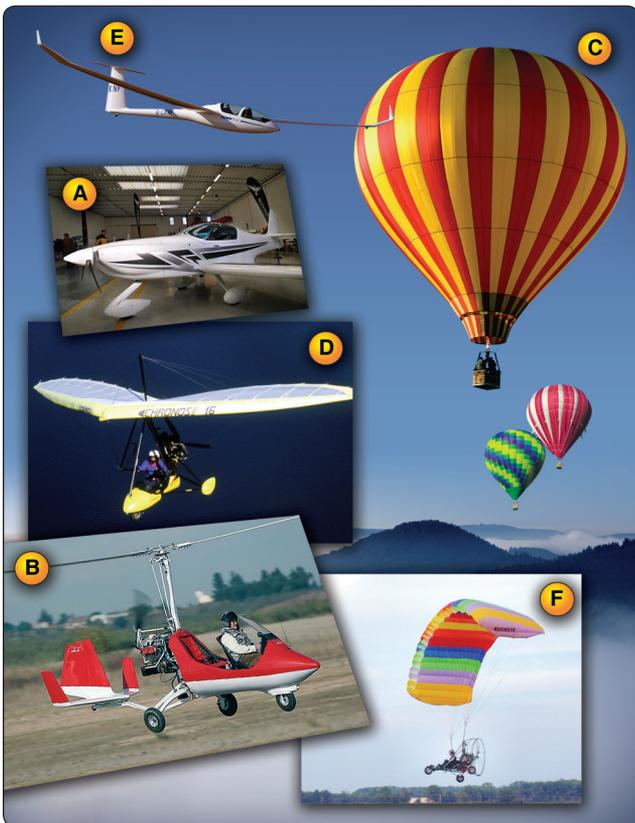
**Figure 16-1.** The LSA category covers a wide variety of aircraft including: A) airplane, B) gyroplane, C) lighter-than-air, D) weight-shift-control, E) glider, and F) powered parachute.
