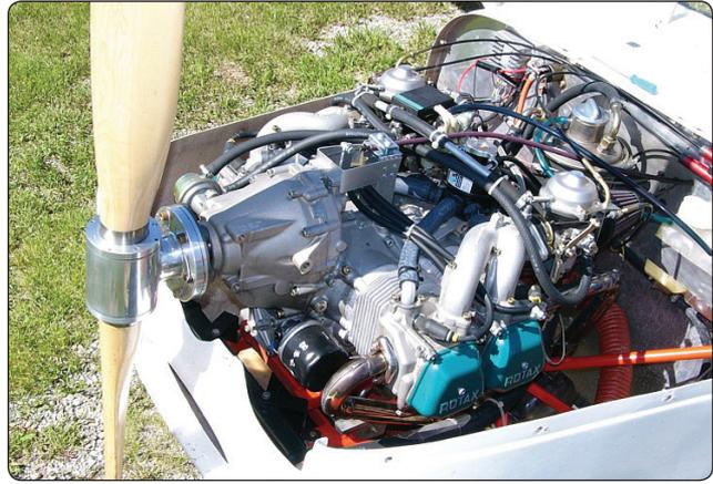
Figure 16-4. A water-cooled 4-cycle engine.
