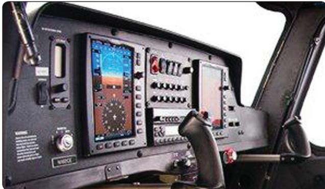
Figure 16-11. *Stoke flight control with conventional engine controls.*
