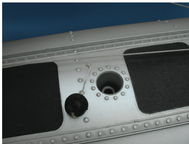
Figure 4-2. Bilge pump openings are closed with a soft rubber ball.
