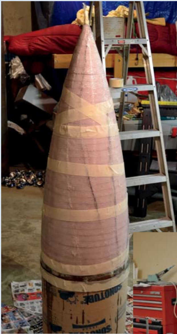
Foam covered in fiberglass to make the nose cone
