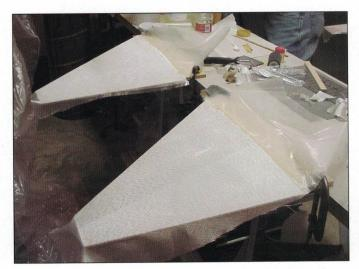
were employed to keep the mess to a minimum. All went well until we got close to the final shape when we picked up a vibration. We then switched to gluing sandpaper onto the template edge and turning the nose by hand, slowly moving the template in until we had the final shape. With the turning complete, we just had to assemble it to see what it looked like. Needless to say, we finally began to realize just how big our project was going to be. It was finally beginning to look like a rock-
