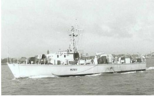
Also one flotilla of Ham Class Inshore 'Sweepers, (164 tons, crew 22), and one flotilla of Underwater Clearance Boats (also Ham Class). The picture on the right is of HMS Bottisham, an example of the Ham Class.
