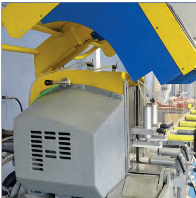
Vortex Tube used to cool saw blade.
