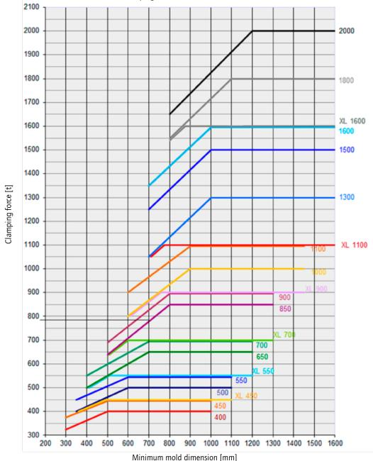
Reductions in clamping force for smaller molds MacroPower
