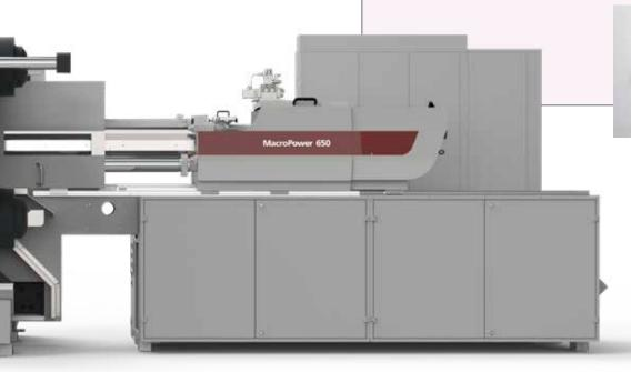
Anti-wear options In addition to the premiumquality standard equipment, an extensive range of options is available to provide extra anti-wear and/or anti-corrosion protection. Predefined option packages and a selection matrix facilitate the selection of the right plasticizing unit.
