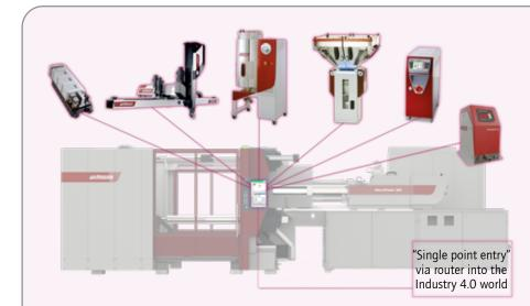
Wittmann 4.0 system With Wittmann 4.0, a machine and its robots and auxiliaries are transformed into a uniform technical organism, which communicates externally via a specific IP address. Such a "single point entry" with an integrated internal firewall substantially increases cyber security.
