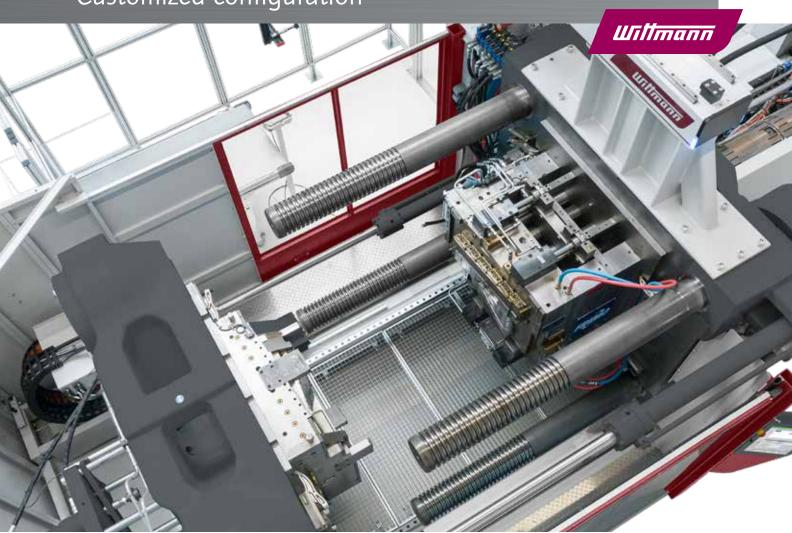
WITTMANN BATTENFELD injection molding machines come with a flexibly adjustable basic modular design. From this basis, the machine can be extended with a wide range of automation equipment into a production cell. This includes primarily devices for fast mold change, fast coupling of complex media connections and the automation of finished parts handling.
