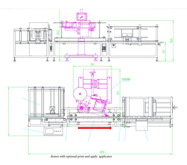
A751LC is a transport platform designed for offline processing of large flat cartons for labeling and inkjet printing. Vertical operation offers the benefits of large capacity supply, labeling and coding on both sides of the flat cartons in the same pass. Inspection system can be added for data verification with optional rejection mechanism.
