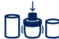
Compression set is the amount by which a compressed elastomeric material fails to return to its original shape when the load is removed. The low compression set of Vulkollan® is a decisive factor behind its successful use for items such as wheels, damping and sealing elements.
