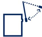
The rebound resilience gives a measure for the elasticity of a material. Vulkollan® shows high and almost constant values over the whole hardness range between 0°C and 120°C. The higher the rebound resilience the less energy is transformed into heat by a deformation.
