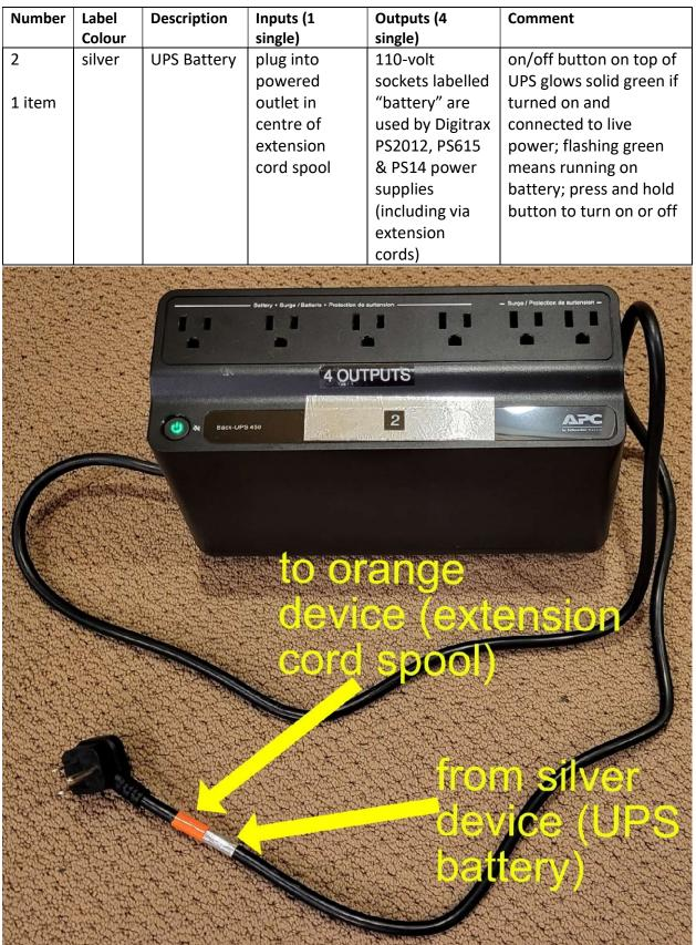
Note colour wire labelling – colour closest to the end of the wire shows which device it plugs into; colour farthest from end of wire shows the device the wire is coming from.
