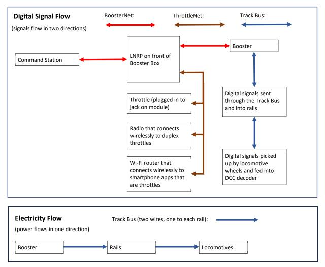
Digital signals are **instructions**: 1) from train operators to the command station; and 2) from the command station to the DCC decoders in locomotives. *Analogy: a TV program is supplied as digital signals sent via a cable or satellite dish.*
