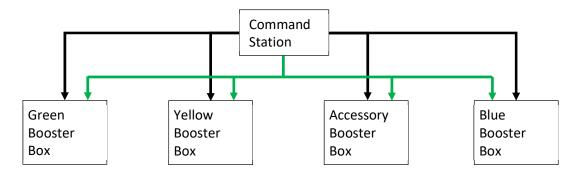
These are the ONLY green cables that need be connected for the entire layout; the green Free-Mo standard cables under the modules should NOT be connected to any of these cables. Connecting these green cables to those under the modules creates a "ground loop" that acts as a large antenna, causing unwanted voltages on the common ground that can cause problems.
