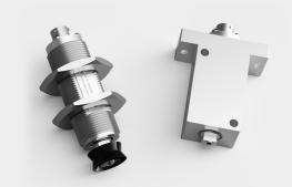
Compact, durable transducers for measuring light tension in fiber, filament or ribbon winding applications. The dual cantilevered beam provides torsional stiffness, strength and accuracy. Available in stackable or threaded through-frame mounting designs.
