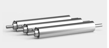
Ultimate performance and robust reliability set the Tension Roll® transducer apart from other sensing solutions on the market. A dead-shaft idler roller with tension sensors (load cells) integrated into each roll end, the Tension Roll® transducer is ideal for installation on original equipment or for retrofits since it arrives pre-assembled and ready-to-install between the facing sides of a machine frame.
