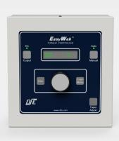
A budget-friendly open-loop controller, the EasyWeb™ calculates the change in roll diameter throughout a winding or unwinding process and adjusts the torque output of your drive, clutch or brake to compensate. This web tension management helps prevent breaking, stretching, wrinkling or curling. The EasyWeb™ uses an input signal from line-speed and roll-speed tachs or from an ultrasonic sensor or rider roll.
