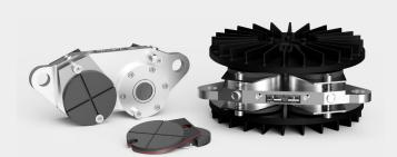
High-output brakes capable of up to 17,990 lb-in of torque. Designed for hassle-free operation, enabling friction pad changes in seconds, without tools. Cylinders can be actuated individually. Piston return springs prevent diaphragm puncture, increasing brake reliability and longevity.
