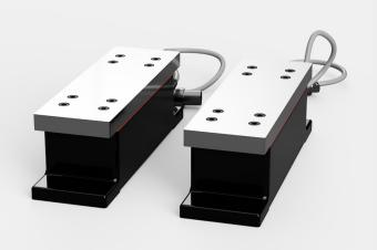
Model F Series transducers mount under pillow-block bearings at each end of an idler roll shaft. Designed for use in demanding tension measurement environments, the F transducer shell has a one-piece aluminum base with a removable stainless steel top plate. A rubber seal between the base and top plate prevents water ingress and dust contamination. The transducer's electrical connector is located at the end of a short cable for simpler access during installation.
