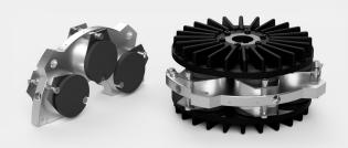
Smaller, high performance dual disk brakes capable of low to moderate torque. Easy to install and use, the 60 series brake was designed for lower tension unwind applications. The 60 series brake can be configured with one to six cylinders.
