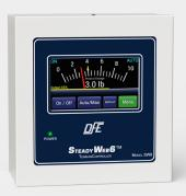
With closed-loop load cell feedback, our flagship SteadyWeb™ 6 tension controller maintains a precise tension setpoint in any zone to improve process consistency. The 5" color touchscreen display simplifies setup and operation.
