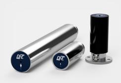
The NW transducer combines a cantilevered idler roll and two tension transducers in one integral unit — for fast, easy installation, high accuracy and web tracking performance. Roll widths from 6" (152 mm) to 20" (508 mm). Choose single-bolt mounting or a four-bolt flange.
