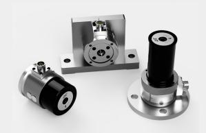
The VNW transducer measures process tension in narrow webs (up to four inches wide), ribbon or filament. It mounts cantilevered on process machinery for unwind/payoff, rewind/take-up, or intermediate zone applications. Robust construction and impressive overload capability.
