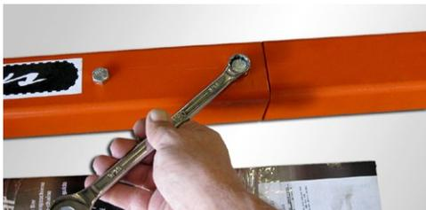
Reinsert the two (2) bolts and tighten with  $\frac{9}{16}$ " wrench to secure.
