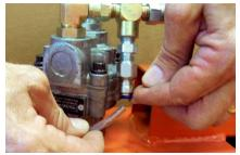
In the event that the preset, self-oiler needs adjustment, remove black outer motor cover to expose oiler. Push up on the blue push lock ring
