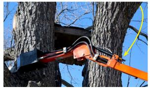
may be necessary to lower your loader to complete a cut. If this is the circumstance, always stop the saw first. Lower your loader until you see the yellow indicator shaft protrude from the back of the shock cylinder again and then resume cutting.
