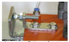
Correct installation and setting of chain tensioner.
