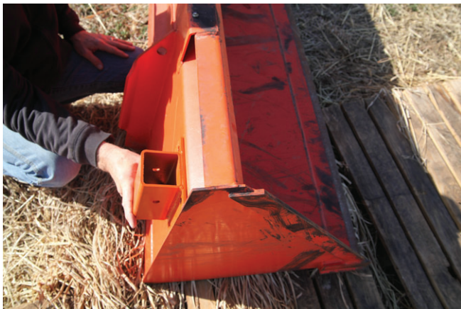
Mounting location of Receiver for VERTICAL CUTS
