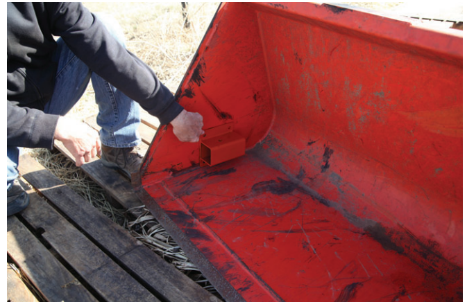
Mounting location of Receiver for HORIZONTAL CUTS
