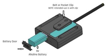
NOTE: Push battery fully into opening before reattaching the battery door
