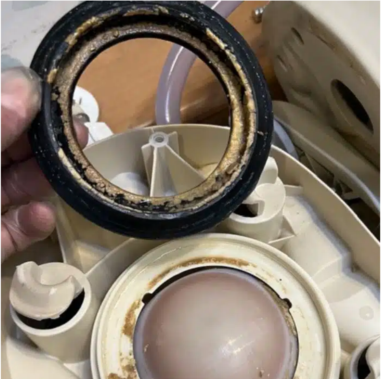
Mineral scale build-up on the seal, waste ball valve, and seal recess.
