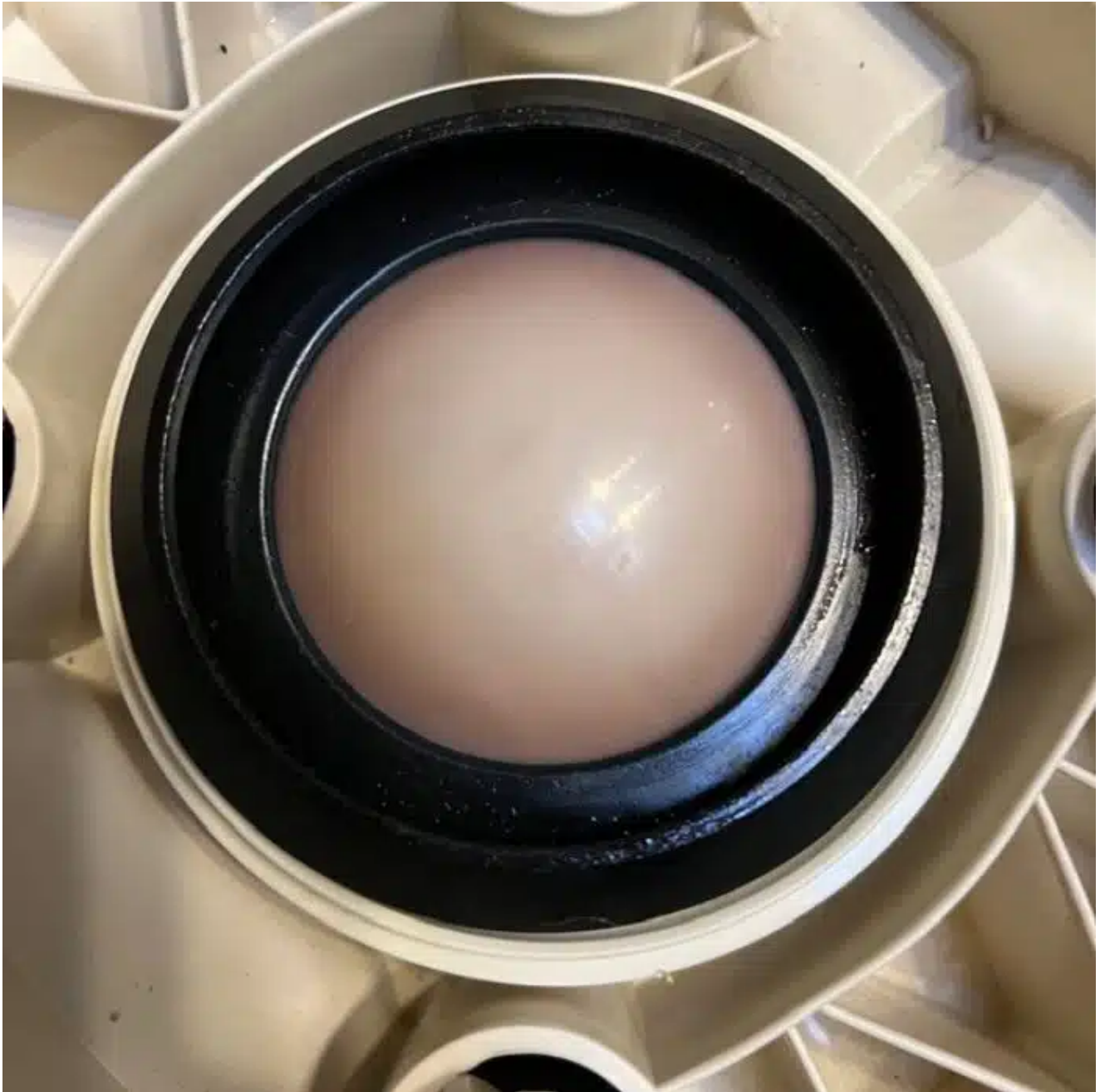
New seal lubricated and placed in seal recess around the waste ball valve
