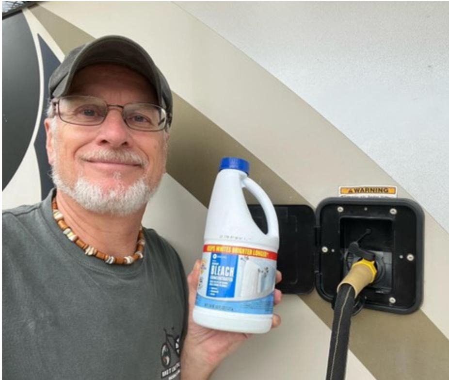
The most common method involves using a diluted solution of  $\frac{1}{4}$  cup of regular chlorine bleach to every 15 gallons of fresh water capacity (Don't use "non-splash/low-splash" or scented bleach, which are not formulated for disinfection purposes). You can mix a small quantity first in a bucket with the full amount of recommended bleach.
