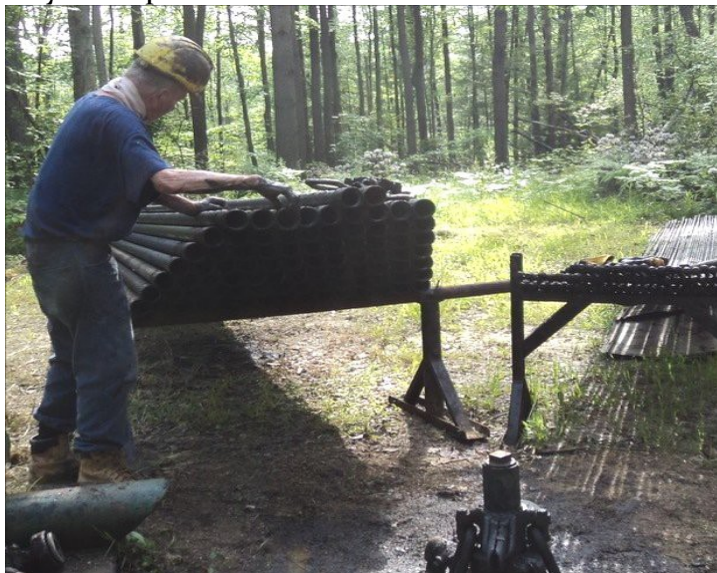
Don Miller on a tubing job at 88. A tubing job is when you first have to pull the rods out and then the tubing, to replace leaky joints or the pump barrel (the two most common reasons).
