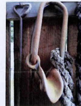
Spudding Shoe - Used to start a new well
