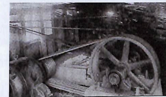
Modern colored power, with V-belt drive, used on a lease near Bradford
