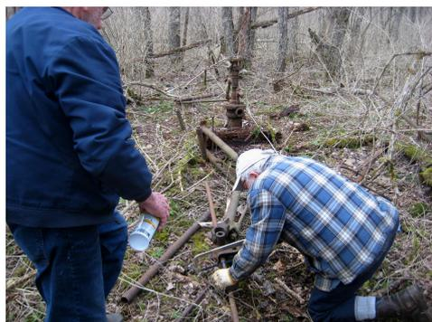
One of the clever features of this jack was that it had an adjustable stroke, from a minimum of 18" to a maximum of 30". The long stroke gave the jack greater pumping capacity and reduced wear on internal parts of the
