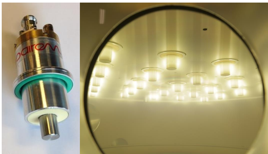
Aura-Wave ECR coaxial plasma source; 25 x 400 W (10 kW), oxygen, 1 Pa
