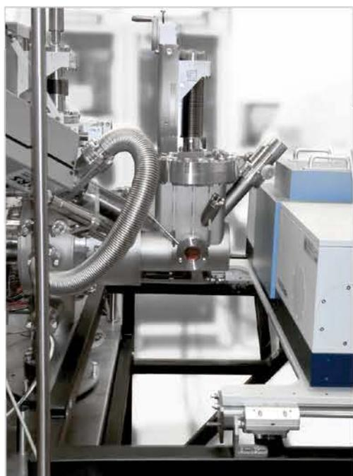
The **IR analyser frame** is independent and can be easily disconnected from the main frame and moved to another position in the laboratory. The system can be extended in the future with the addition of other chambers or techniques e.g. MBE.
