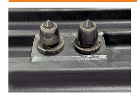
A steel block is installed between the lugs of the track which is permanently welded in place. Studs are then inserted into the blocks
