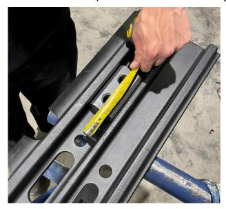
**Step 2:** Place the block on track over the pre cut holes and weld beveled edges to the lugs. The block being permanently fixed should now be flush with the top of the track lugs.
