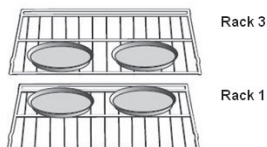
Multiple rack pan placement
