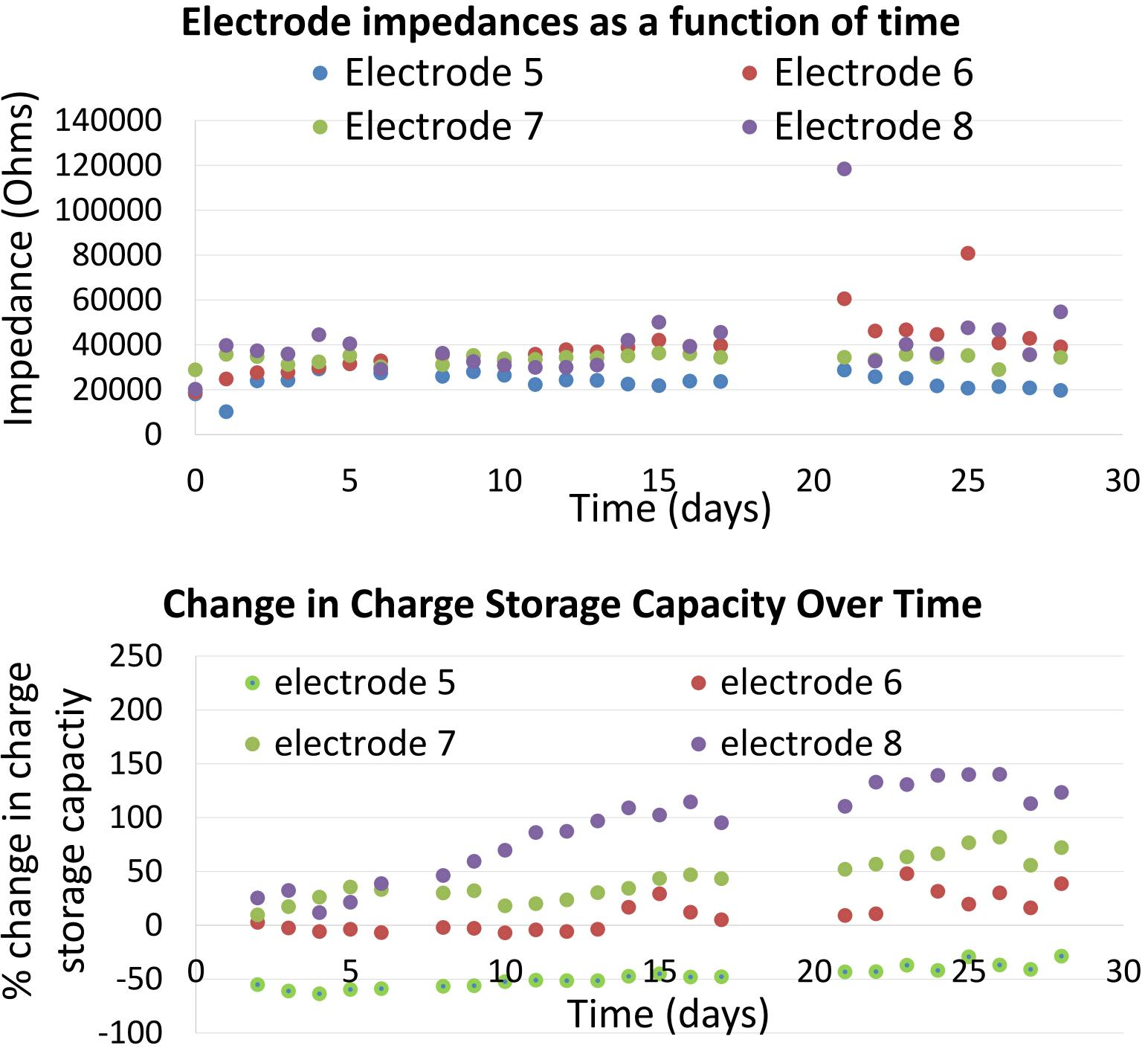
**Figure 3**: Typical impedances at 1 kHz (top) and charge storage capacity (bottom) in an array over the duration of a chronic experiment show no significant changes.
