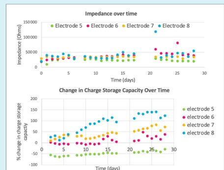
Figure 3: Typical impedances at 1 kHz (top) and charge storage capacity (bottom) in an array over the duration of a chronic experiment show no significant changes
