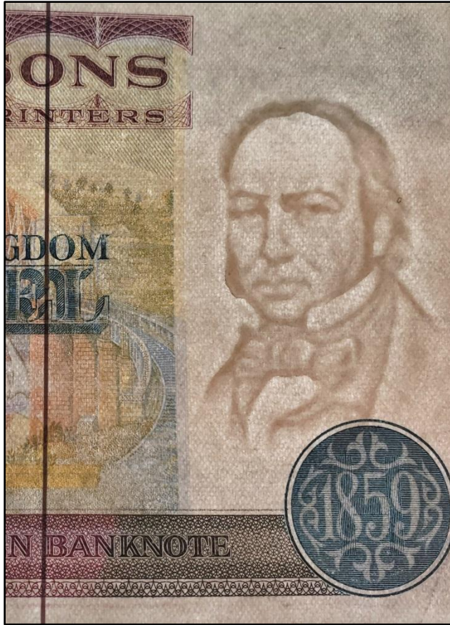
Figure 4 Back light image showing watermark & security strip
