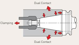
Taper Dual Contact Spindle
