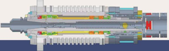
The rigid spindle reduces vibration to ensure greater accuracy
