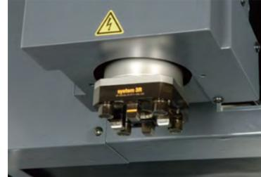
Supports parallel electrode setup and index machining
