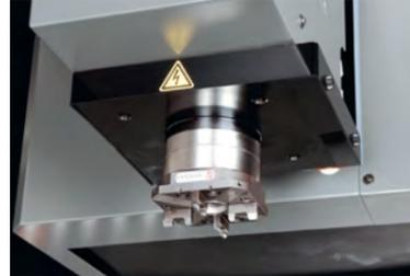
Clamp spindle side holder with air chuck
