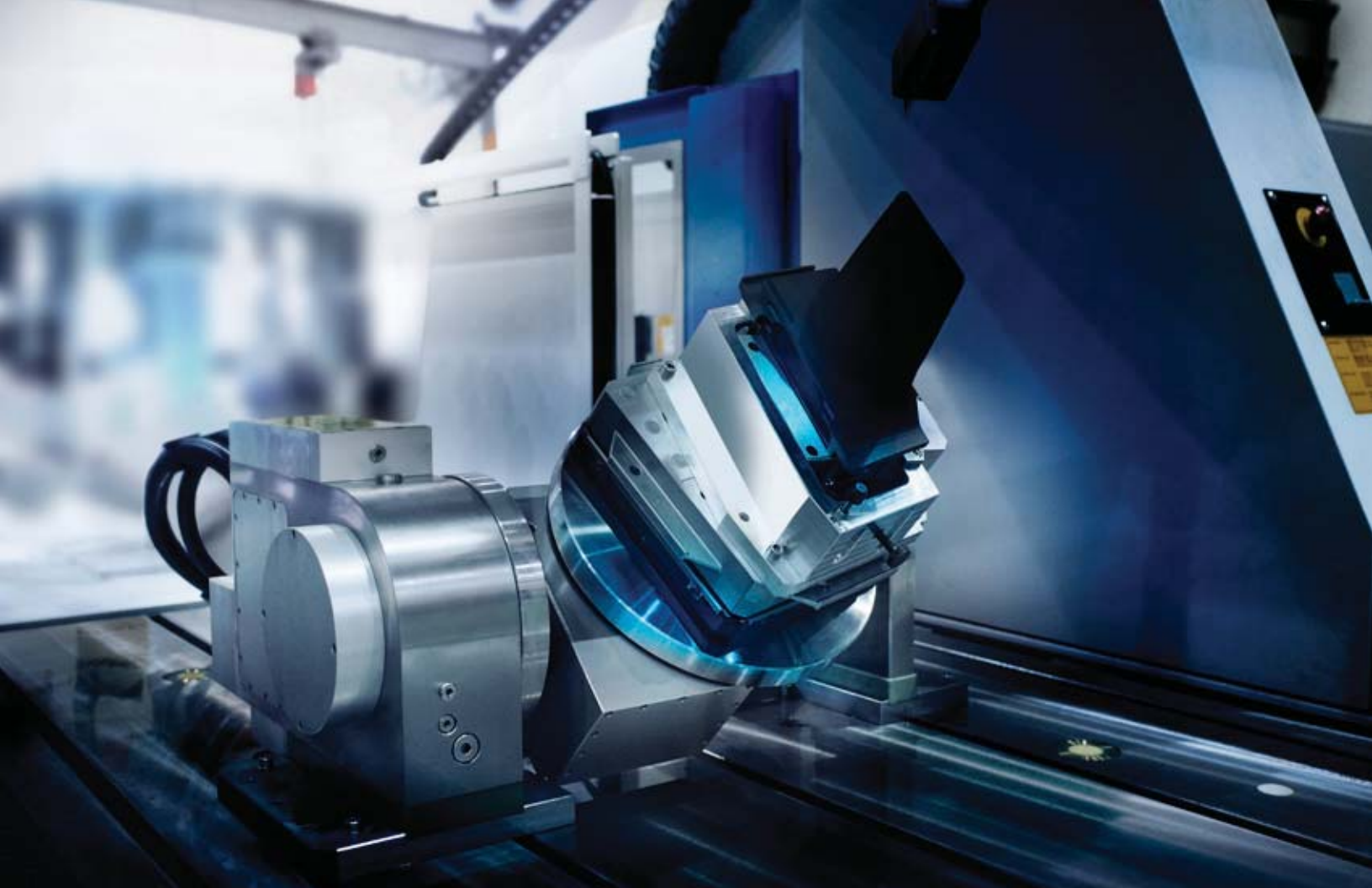
5 th /6 th axis as a fully integrated EDM axes for machining high-precision components of different sizes
