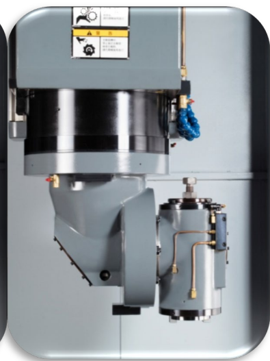
30 Degree, 3000 RPM 1:1.16 Gear Ratio
