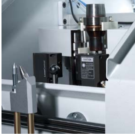
Measuring laser in the tool changer
