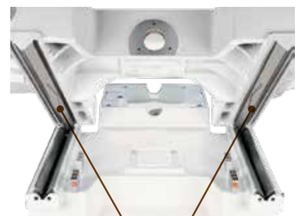
Cross feed double "V" guideways
