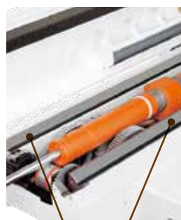
Longitudinal double "V" guideways
