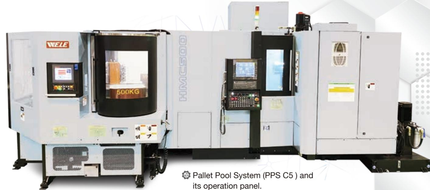
⚙️ Pallet Pool System (PPS C5) and its operation panel.
