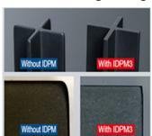
IDPM3 automatically adjusts the spark to reduce the electrode wear while optimizing machining speeds with graphite electrodes.
