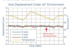
Machining accuracy is improved through a Thermal Displacement Compensation system and Z-Axis cooling mechanism.
