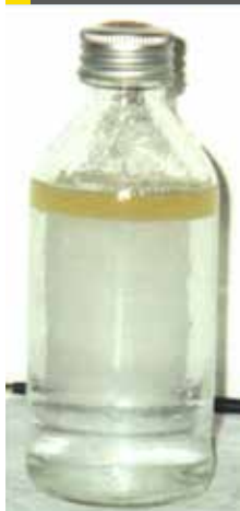
Fig 6: Foaming tendency of hydrocarbon contaminated amine
