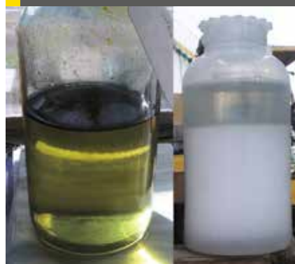
Fig 11: Reflux water with skimmable hydrocarbon
