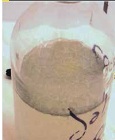
Fig 6: Foaming tendency of hydrocarbon contaminated amine
