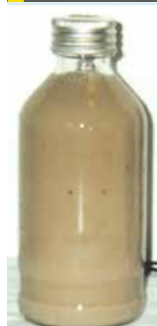
Fig 6: Foaming tendency of hydrocarbon contaminated amine
