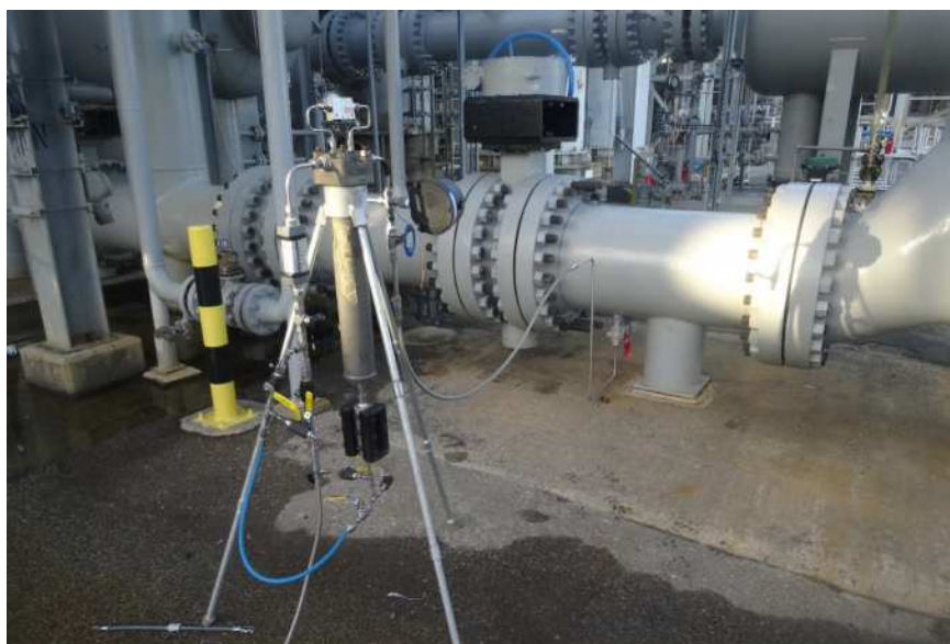
Figure 1. GASCO sampling unit as assembled for feed gas contamination testing and sampling.
