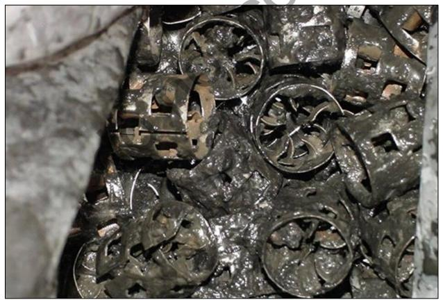
FIG. 2. Deposits by suspended solids in column pall ring packing.
