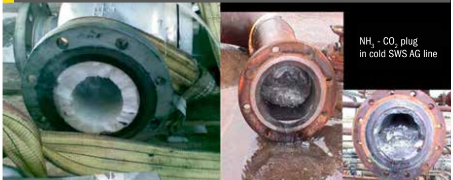
Fig 6: Ammonium salt sublimation
