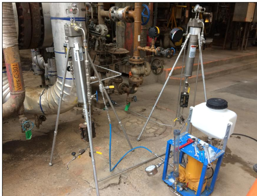
**Figure 5** GASCO test units in operation for sampling feed LPG upstream of the amine unit contactor
