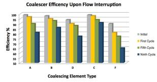
Figure 5. This graph shows the effect of gas flow interruption on different gas-liquid coalescing elements.
