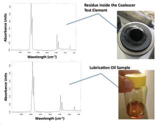
Figure 4. These photos and associated IR spectra illustrate residue from the GASCO test element.
