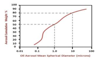
Figure 3. This shows a typical liquid aerosol size distribution at the outlet of a compressed gas stream.
