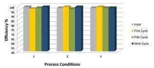
Figure 6. This graph shows the effect of gas flow interruption on the XC gas-liquid coalescing element.
