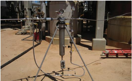
■ Figure 2. The photo shows the setup of the GASCO test system for a compressed gas stream.
