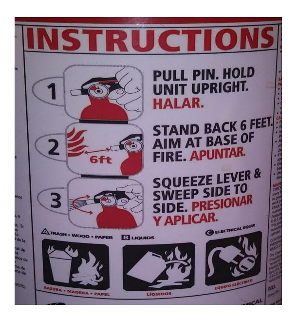
See picture for proper instructions on how to use a fire extinguisher.
