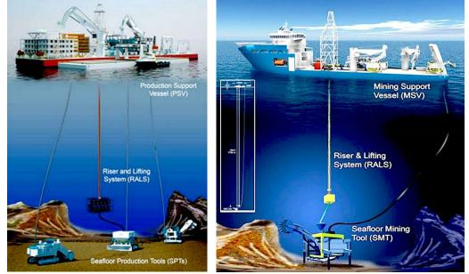
The subsea mining will be done with ships and robotic tools like the ones in pictures below.
