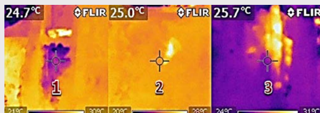
AFTER 45 MINUTES WITH EP-2 MIXED IN 11% HEAT REDUCTION
